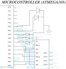
The ATmega168 microcontroller is used to process the signal obtained from the proximity sensors. The advantage of using this is we can convert the analog signals to digital signals for the controlled motion. This is programmed such that depending upon the signal obtained from the sensors the microcontroller sends signals having the changes that have to be performed by the slave in order to maintain it in the area of vicinity.
