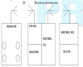
The wireless remote controls the master by sending some signals, and hence the master is controlled manually. The master performs actions as per the remote instructions. For every change in master's direction the slave performs some action. We use IR radiations for controlling the master and RF signals to control the slave.
