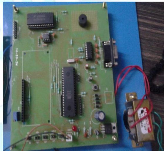
**Cluster node 2:** Dc gas control system is the second cluster node for this experiment. It includes mq-6 gas sensor, Adc for data acquisition and pic as controller. The objective of this dc motor is to control the gas at certain threshold level.
