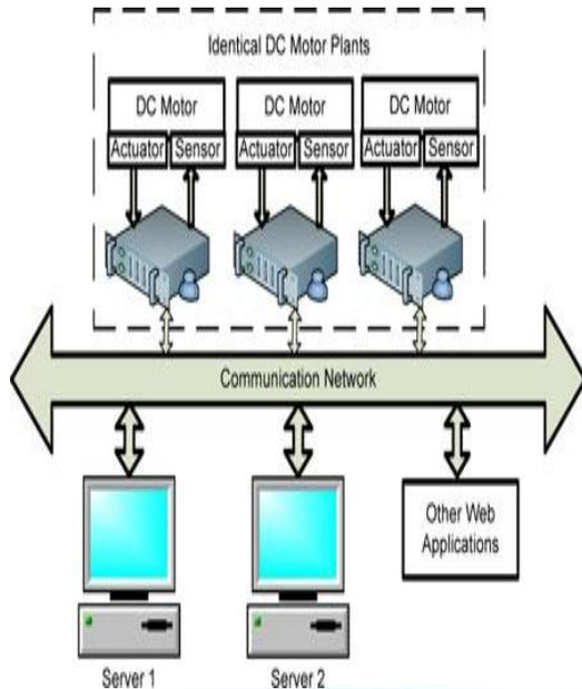
**BLOCK DIAGRAM FOR MULTI-CLIENT- SERVER ARCHITECTURE**
