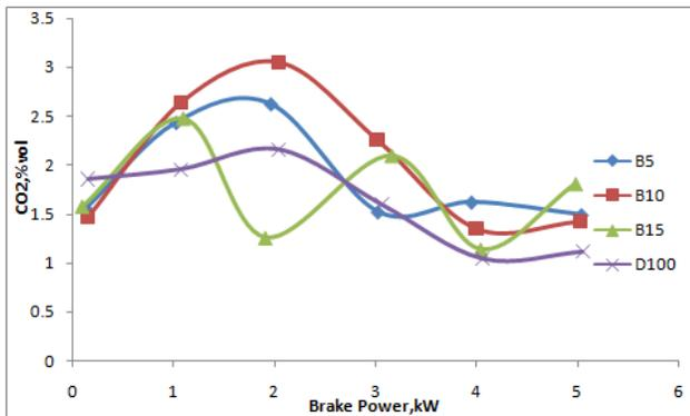
Fig 9 Variation of carbon dioxide with brake power
