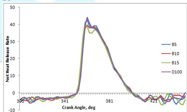
Fig 12 Show the variation of net HRR with crank angle
