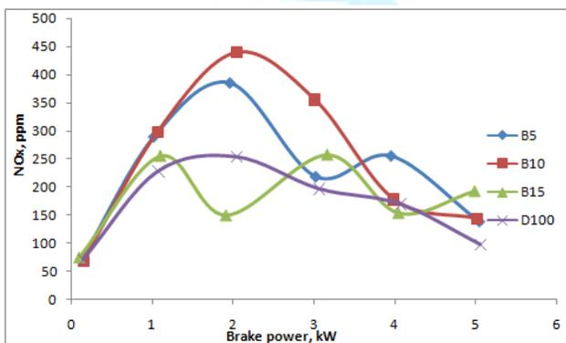
Fig 10 Variation of NOx with brake power
