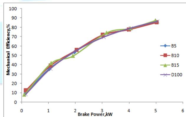
Fig 4 Variation of mechanical efficiency with respect to brake power
