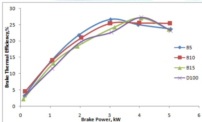
Fig 2 Variation of brake thermal efficiency with respect to brake power
