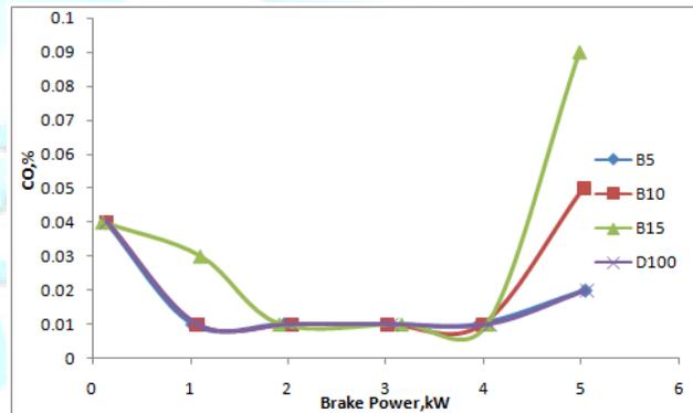
Fig -7: Variation of carbon monoxide with brake power
