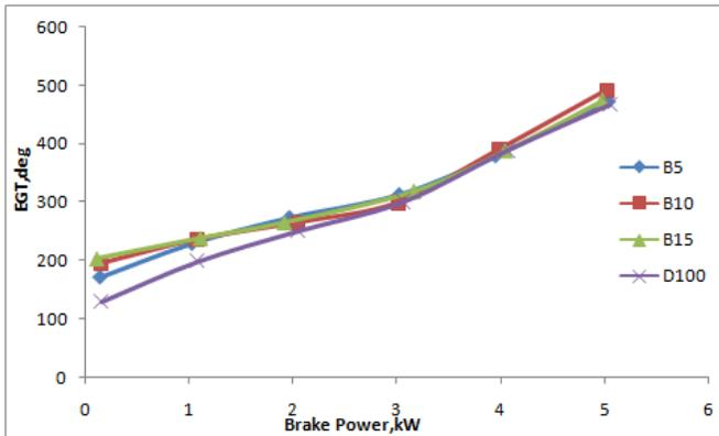
Fig 5 Variation of exhaust gas temperature with respect to brake power
