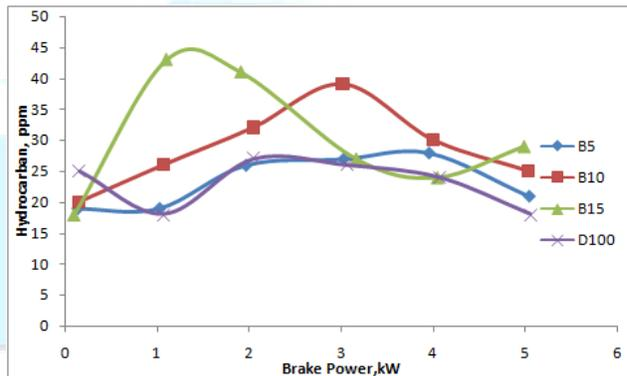
Fig 8 Variation of HC emission with Brake power
