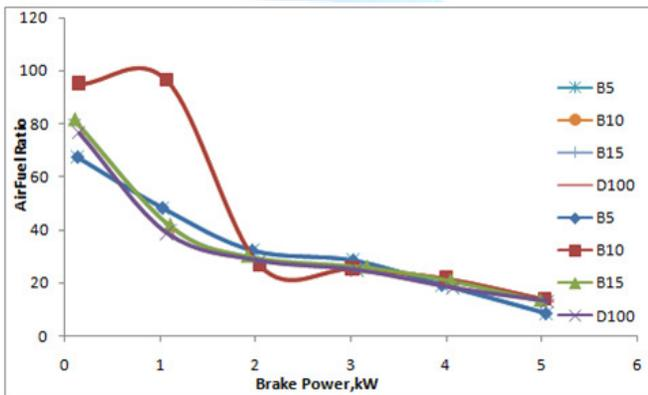
Fig 6 comparison of A/F ratio with respect to brake power
