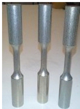
Fig. 4. The test parts made of SS 420 + Bronze
