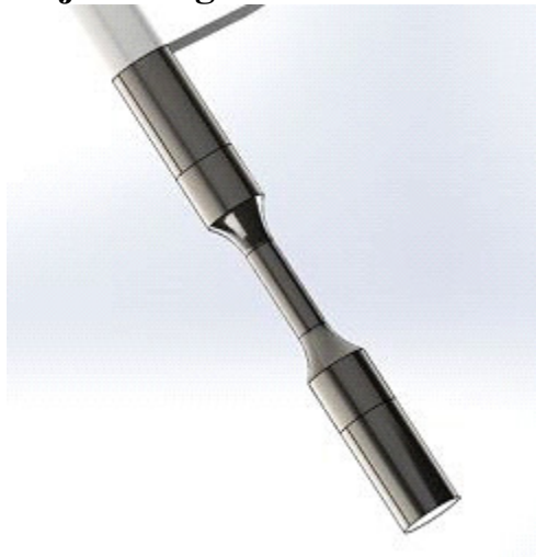
Fig. 2 The 3D computer model of the fatigue test part.
