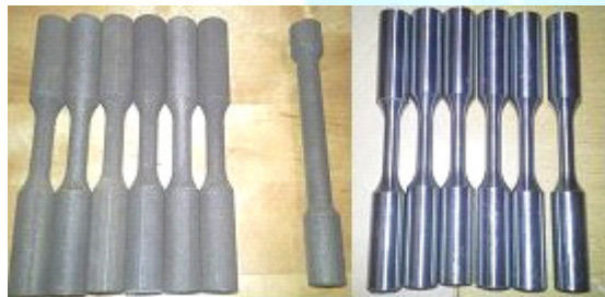
Fig. 3 The test parts made of EOS 316 L.
