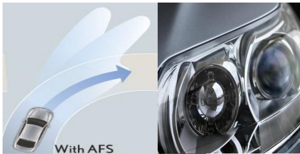
Fig 5: a) light pattern aiming to achieve (b) head lamps to be used in proposed design
