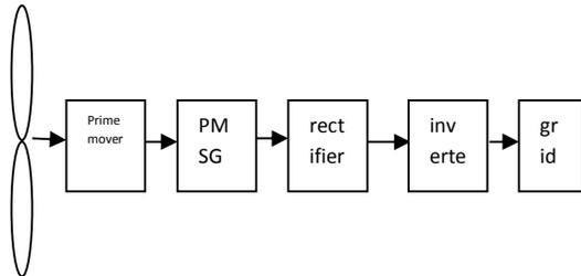
Fig.1 generalized block diagram of wind energy conversion system
