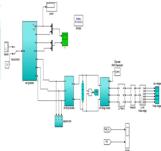
Fig.5.1 MATLAB/SIMULINK model of WECS
