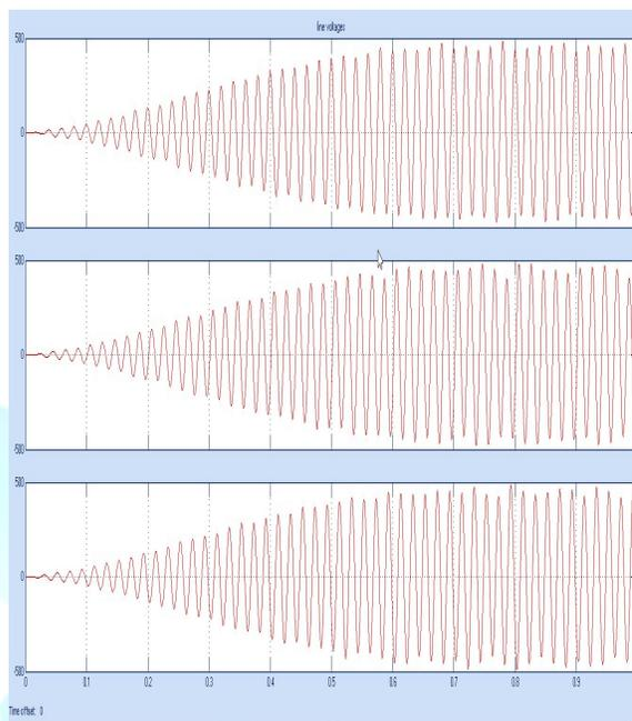
Fig.4.3(c) line voltage at grid side without harmonic
