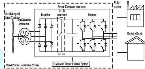
Fig.2.1 layout of PMSG based on WECS
