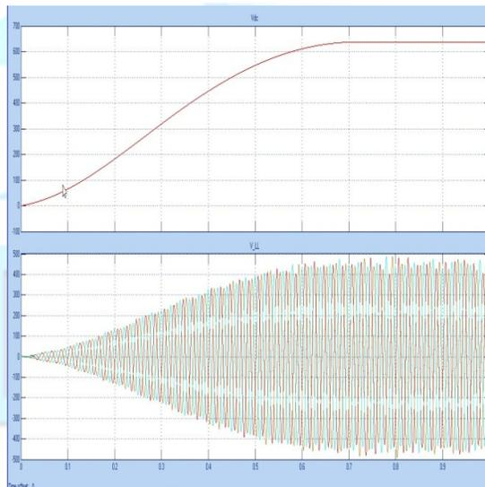
Fig.4.4 (d) voltage at inverter and rectifier side with DC link Capacitor, LC filter
