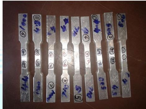
Figure 3. shows the tensile specimen used.
