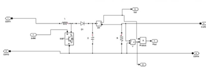
Fig4. Circuit of dc-dc boost converter
