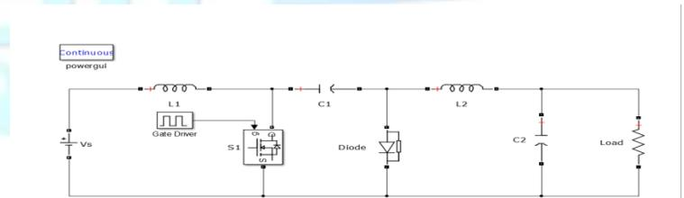
Fig5. Circuit of dc-dc CUK converter
