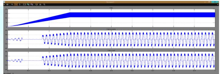
Fig.15 Voltage at DC bus, inverter and at load
