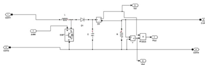
Fig4. Circuit of dc-dc boost converter
