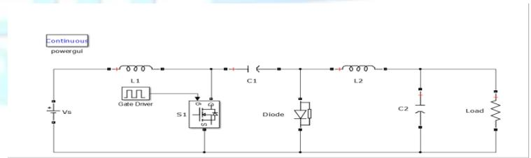
Fig5. Circuit of dc-dc CUK converter
