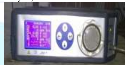
Fig 10 : Photographic view of Exhaust Gas Analyzer
