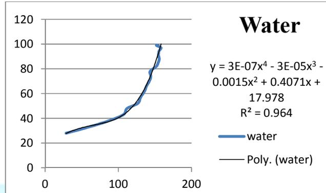
Fig 3.6 Inside temp (Water) v/s Outer surface temp of vessel
