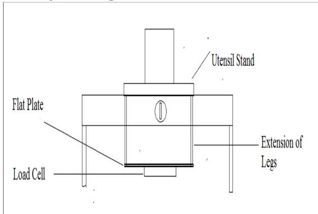
Fig 5.3 Load cell setup
