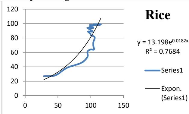
Fig 3.3 Inside temp (rice) v/s Outer surface temp of vessel
