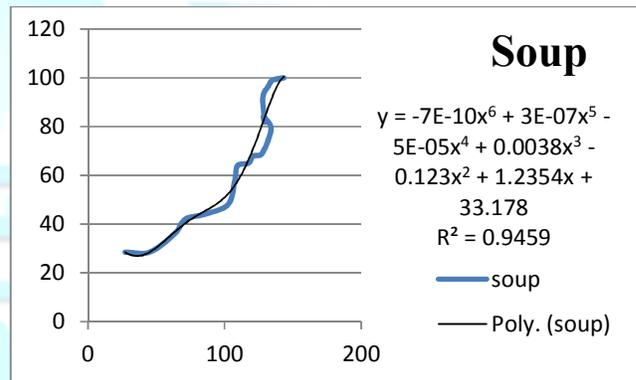
Fig 3.7 Inside temp (Soup) v/s Outer surface temp of vessel
