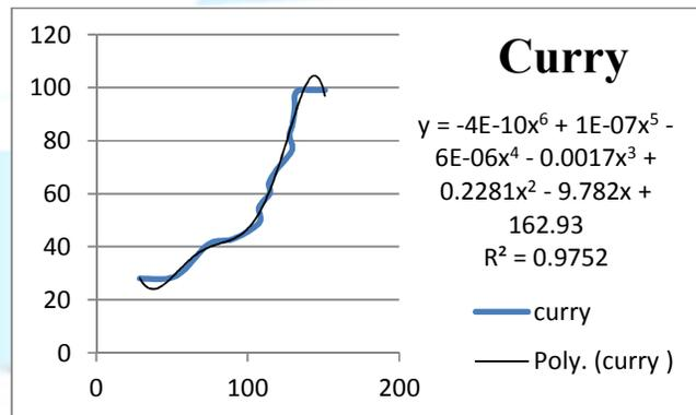
Fig 3.8 Inside temp (Curry) v/s Outer surface temp of vessel
