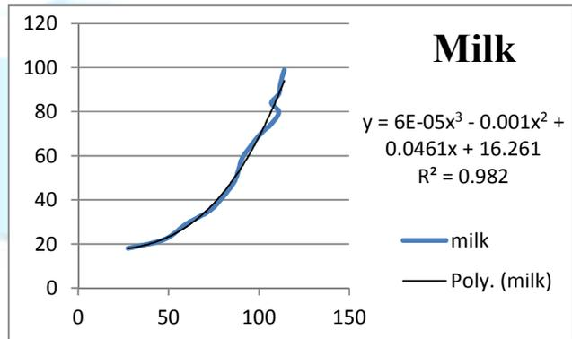
Fig 3.2 Inside temp (milk) v/s Outer surface temp of vessel
