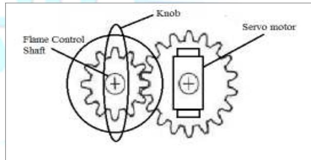
Fig 5.2 Flame control mechanism
