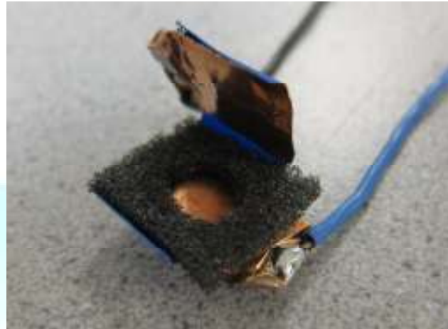
Fig. 3 Contact pad Sensor
