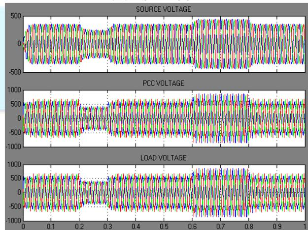
Fig. 8. Source, PCC and load voltages in PFI mode with one DSTATCOM
