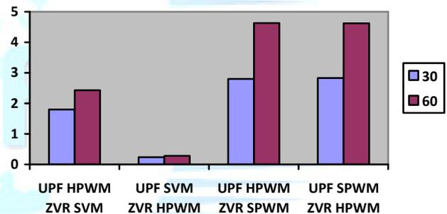
Fig 15. THD value of phase-A source current with two DSTATCOMs
