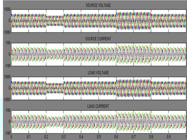
Fig. 6. Waveforms without DSTATCOM
