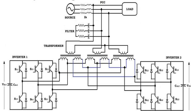
Fig. 5 Two DSTATCOMs connected to a three-phase three-wire distribution system
