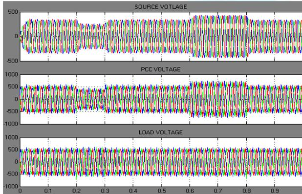
Fig 10. Source, PCC and load voltages in VR mode with one DSTATCOM
