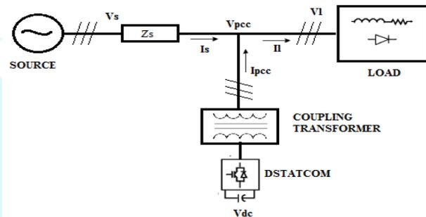
Fig. 1 Basic layout of DSTATCOM.
