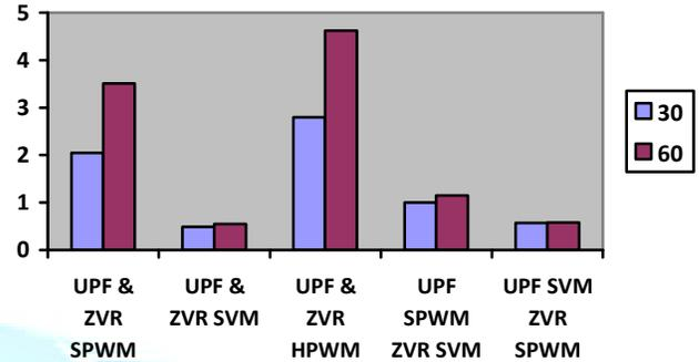
Fig 14. THD value of phase-A source current with two DSTATCOMs
