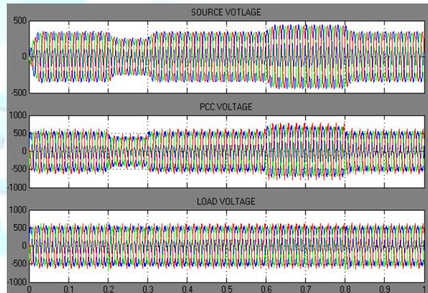
Fig 12. Source, PCC and load voltages with two DSTATCOMs
