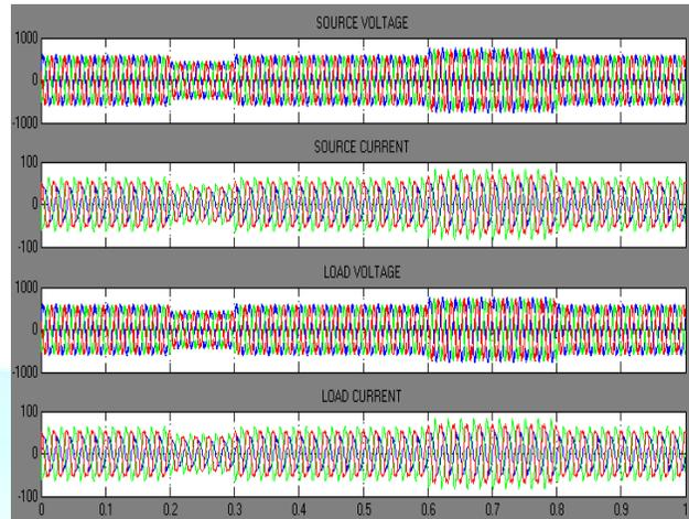
Fig. 6. Waveforms without DSTATCOM
