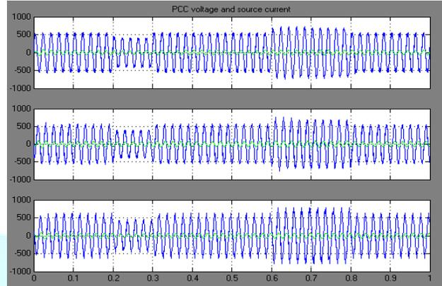
Fig 11. PCC voltage versus source current with two DSTATCOMs
