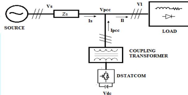
Fig. 1 Basic layout of DSTATCOM.
