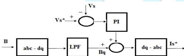
Fig. 3 Voltage regulation block diagram.
