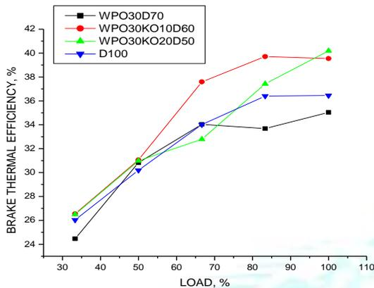
Fig. 2 Variation of Brake Thermal Efficiency with load
