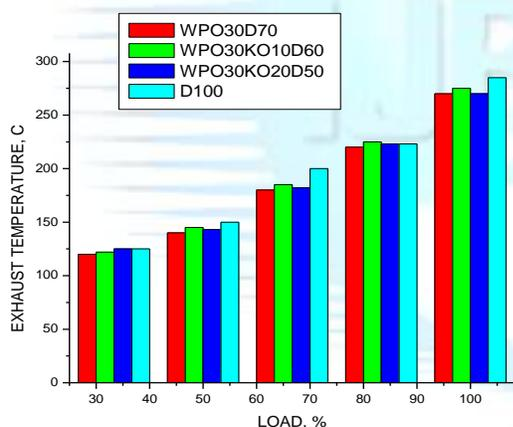
Fig. 6 Variation of Exhaust Temperature with Load
