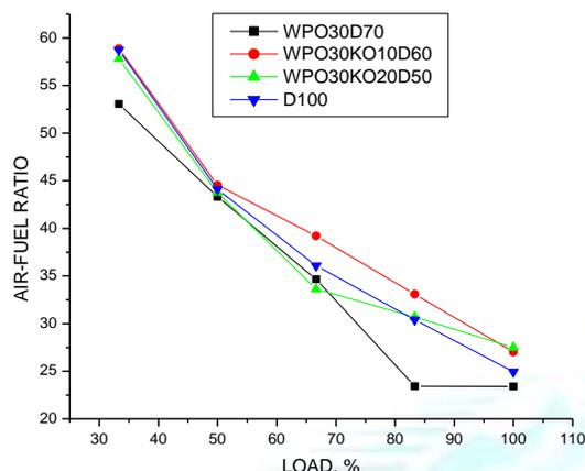
Fig. 5 Variation of Air- Fuel Ratio with Load
