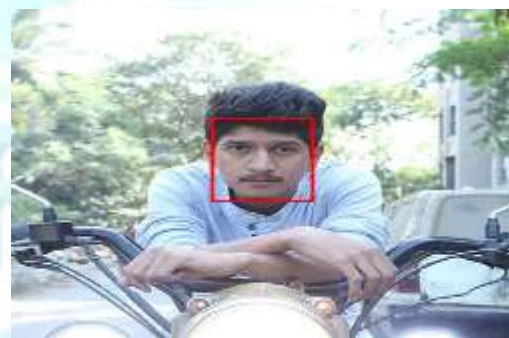
Figure 5: After applying face detection with OpenCV.
