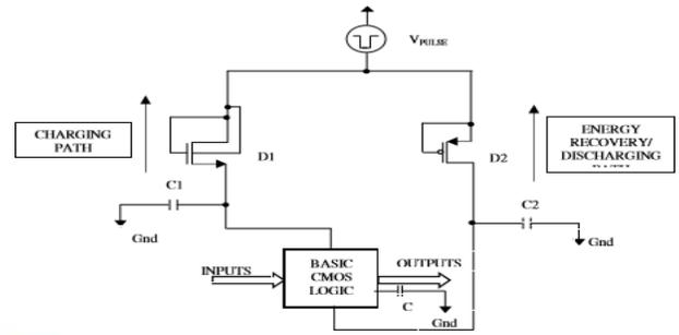
Fig 5b Basic circuit using adiabatic gate
