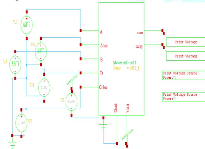
Fig: 6a Schematic of proposed Full Adder
